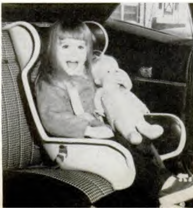
SIDE PROTECTION is given by Klippan Safety Auto Seat for kids up to about 42 inches and 50 pounds
